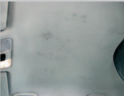
Excessively soiled headlining that cannot be removed by normal cleaning. Also unacceptable are any tears in the material.
