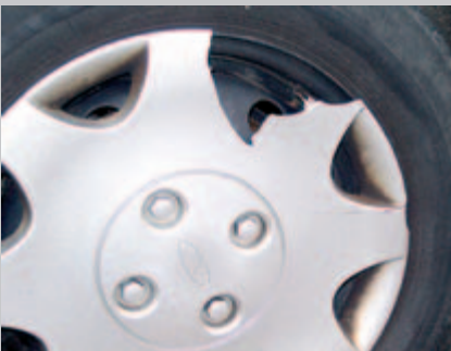
Deformed wheel trims due to breakages or scuffing. Cracks or breaks to the trim. Missing trims.
