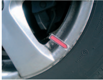
Scuffing, scratches or deposits on rims, if the rim is not deformed.
