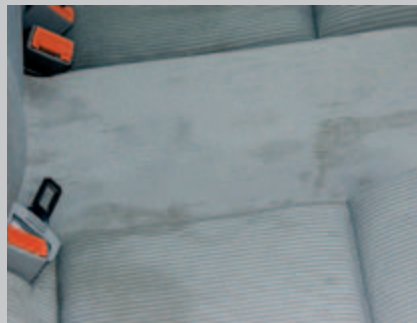
Excessive soiling and dirt which cannot be removed by general cleaning.
