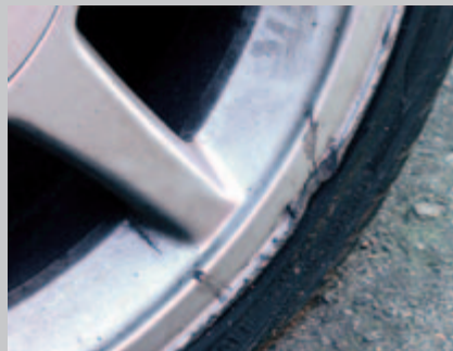
Rims with heavy damage, deformation of the rim or missing parts.
